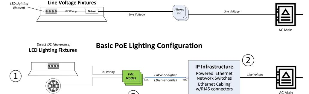
Ethernet cables replace AC line voltage runs and provide low voltage DC power from Powered Ethernet Network Switches and connectivity for device control and integration via palm-sized, proprietary PoE Nodes
