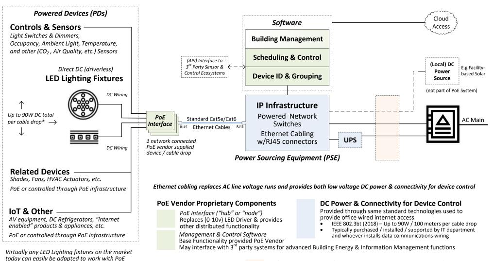
\* Per current IEEE standard. Practical limit when specifying actual loads is 71W total per cable drop. DC/Alternative Building / Campus Power Infrastructure (Optional / Future) Lighting is typically 40% of building electricity usage. eliminating the need to power lights with AC electricity is a significant step towards making DC & other Power Infrastructure options feasible
